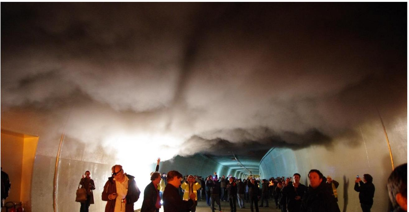
Nick recently attended a hot smoke test in Marseille, France where potassium nitrate and starch were used to generate both heat and smoke. The flow visualisation objectives were met quickly and simply. Photos of that test are below.
