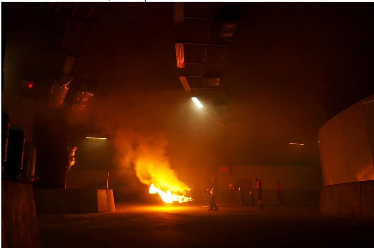
The other characteristic of LPG burners is that the heat release may be much more concentrated than for a general fire, giving a faster initial plume rise. The perception by some that LPG flames were not 'realistic' led us to develop the RDP (photo below). The vehicle shell is simply a diffuser for the plume at source.
