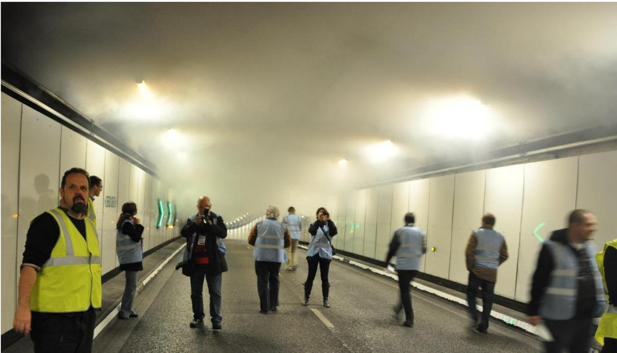
Combining 200 kW of LPG heaters and electric smoke generators, we recently conducted a flow visualisation test in a bus station. That methodology, the results of which are shown below, allowed for six detailed response mode tests to be conducted over a period of two and a half hours. This test methodology, perhaps using a higher heat release rate, would be well-suited to road tunnels.
